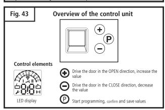
For proper initial operation of the operator, three basic functions must be set using the initial system programming:
