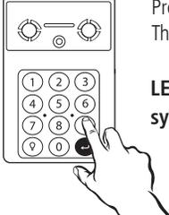
To test, enter the temporary PIN, then press the ENTER button. The garage door operator will activate. If the temporary PIN was set for a number of openings, the test will use up one opening programmed PIN.
